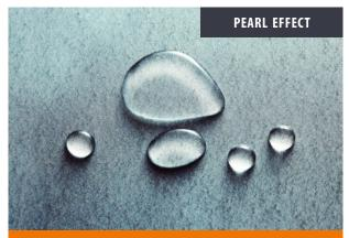
Surface resistance to wetting as water beads are repelled. Water droplets bead on the surface "they are not absorbed" but roll down the facade washing away dirt and dust.
